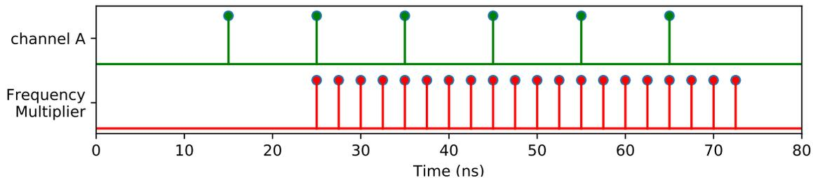
Frequency Multiplier for a channel with a periodic signal.
