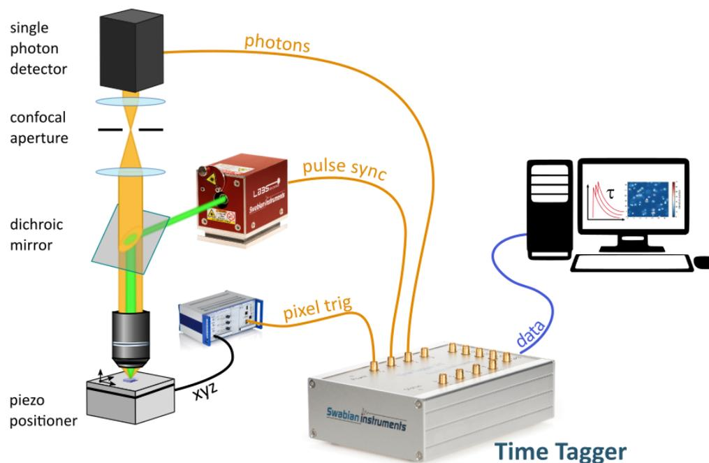
In this setup, the objective focuses the excitation light from the laser at the fluorescent sample and, at the same time, collects the resulting emission. The emission photons pass through the confocal aperture and arrive at the single-photon detector (SPD). For every detected photon, the SPD produces a voltage pulse at its output, namely a photon pulse.
