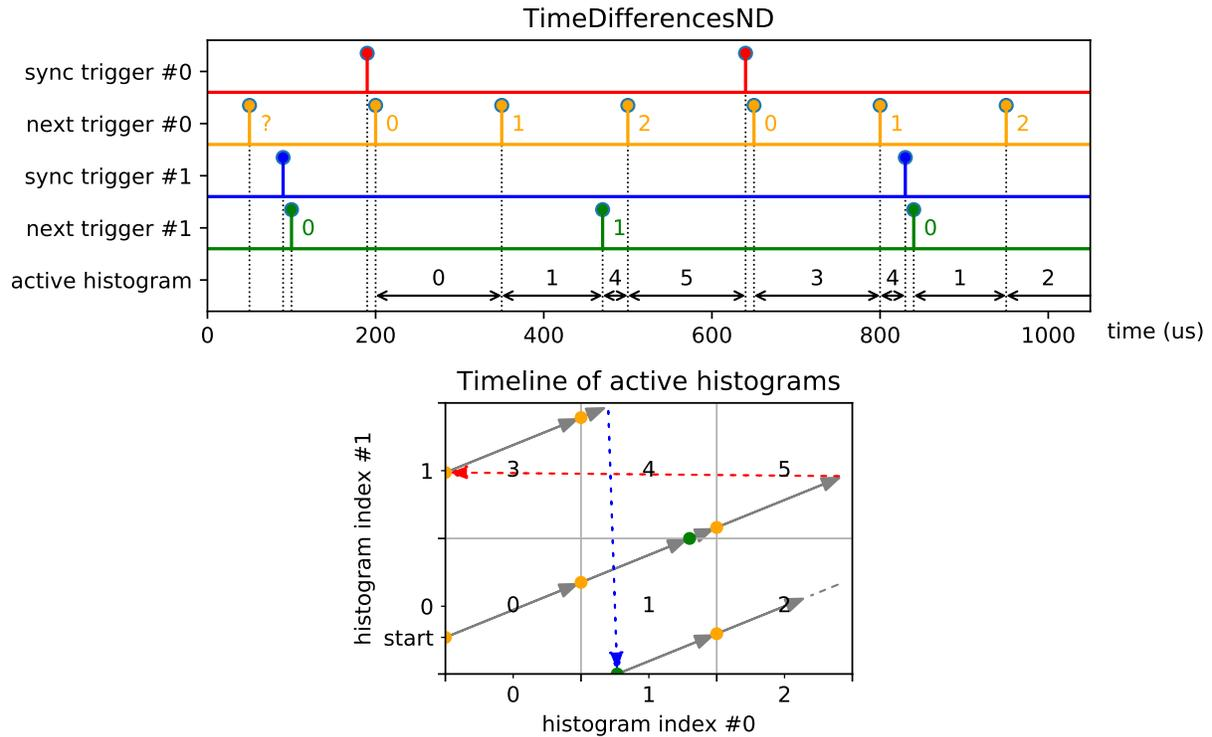
This is an implementation of the *TimeDifferences* measurement class that extends histogram indexing into multiple dimensions.
