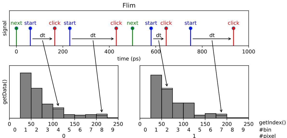
Fluorescence-lifetime imaging microscopy (FLIM) is an imaging technique for producing an image based on the differences in the exponential decay rate of the fluorescence from a sample.
