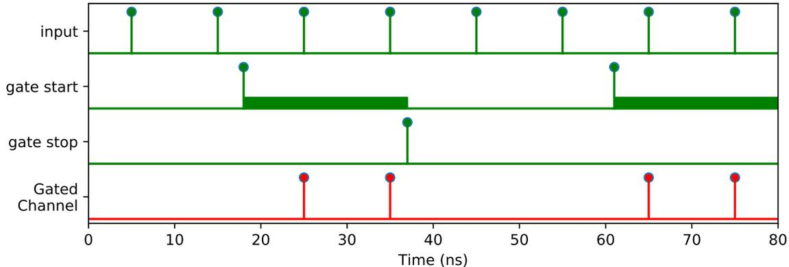
Transmits the signal from an `input_channel` to a new virtual channel between an edge detected at the `gate_start_channel` and the `gate_stop_channel`.
