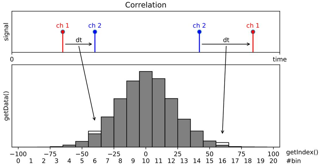
Accumulates time differences between clicks on two channels into a histogram, where all ticks are considered both as “start” and “stop” clicks and both positive and negative time differences are considered.
