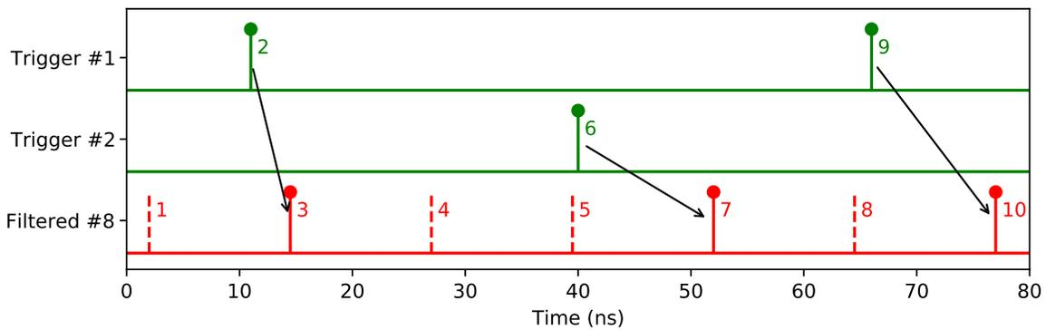
This is the typical use case when you detect photons with multiple detectors and want to correlate both with the common excitation laser.
