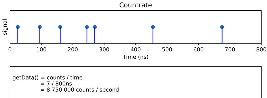
Measures the average count rate on one or more channels. Specifically, it determines the counts per second on the specified channels starting from the very first tag arriving after the instantiation or last call to `clear()` of the measurement. The `Countrate` works correctly even when the USB transfer rate or backend processing capabilities are exceeded.
