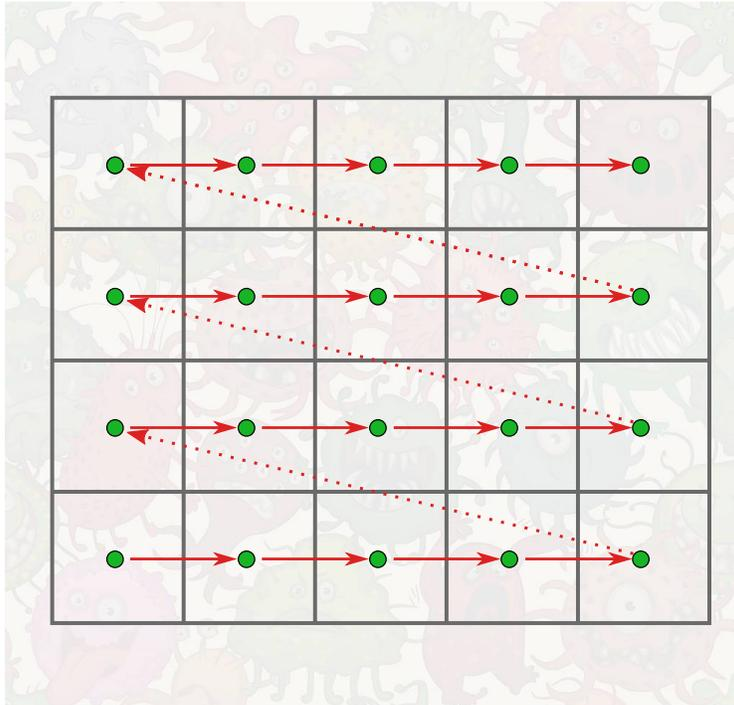
In the figure above, the scan starts from the bottom-left corner and proceeds horizontally in steps. At each scan position, the scanner has to wait for arbitrary integration time to allow sufficient photon collection. This process stops when the scanner reaches the top-right point.
