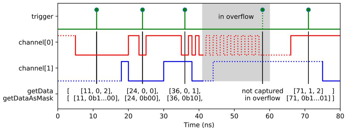
The *Sampler* class allows sampling the state of a set of channels via a trigger channel.
