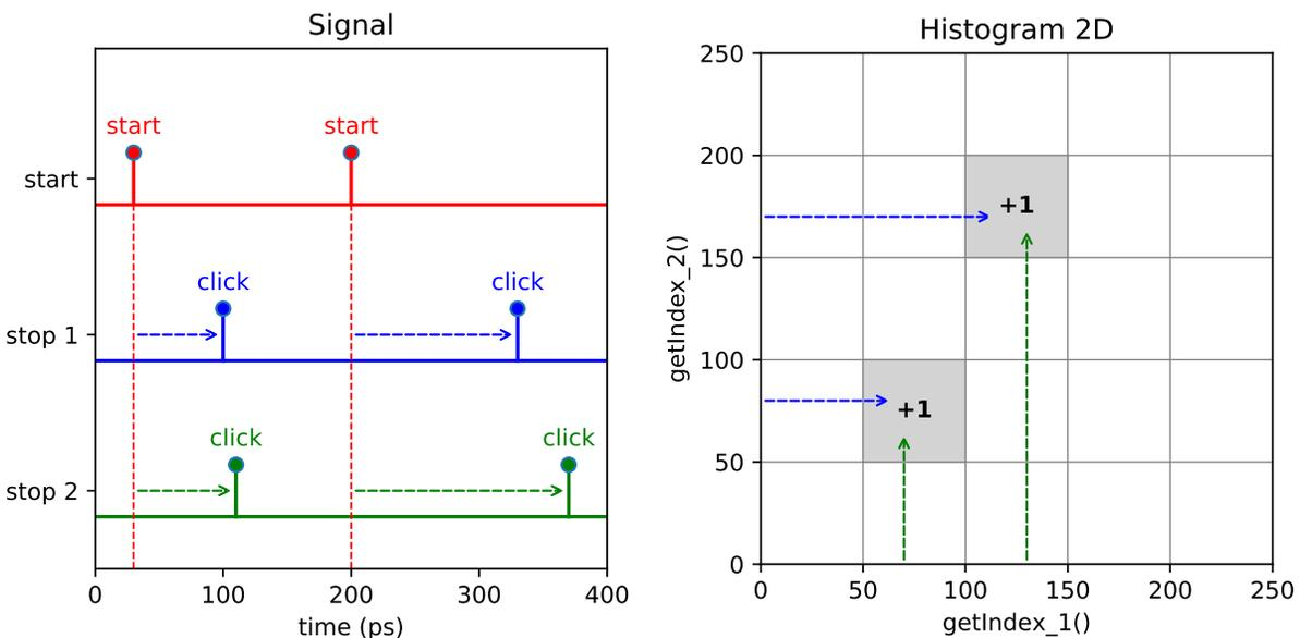
This measurement is a 2-dimensional version of the *Histogram* measurement. The measurement accumulates a two-dimensional histogram where stop signals from two separate channels define the bin coordinate. For instance, this kind of measurement is similar to that of typical 2D NMR spectroscopy. The data within the histogram is acquired via a single-start, single-stop analysis for each axis. The first stop click of each axis is taken after the start click to evaluate the histogram counts.
