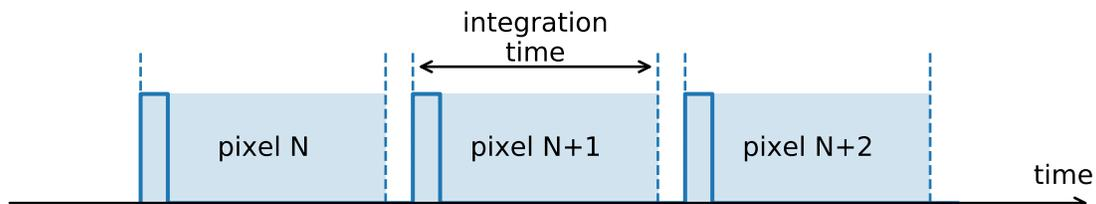
When a pixel pulse has a duration different from the desired integration time, we must define the integration time manually. One way would be to record all events until the next pixel pulse and rely on a strictly fixed pixel pulse period. Alternatively, we can create a well-defined time window after each pixel pulse, so the measurement system becomes insensitive to the variation of the pixel pulse period.
