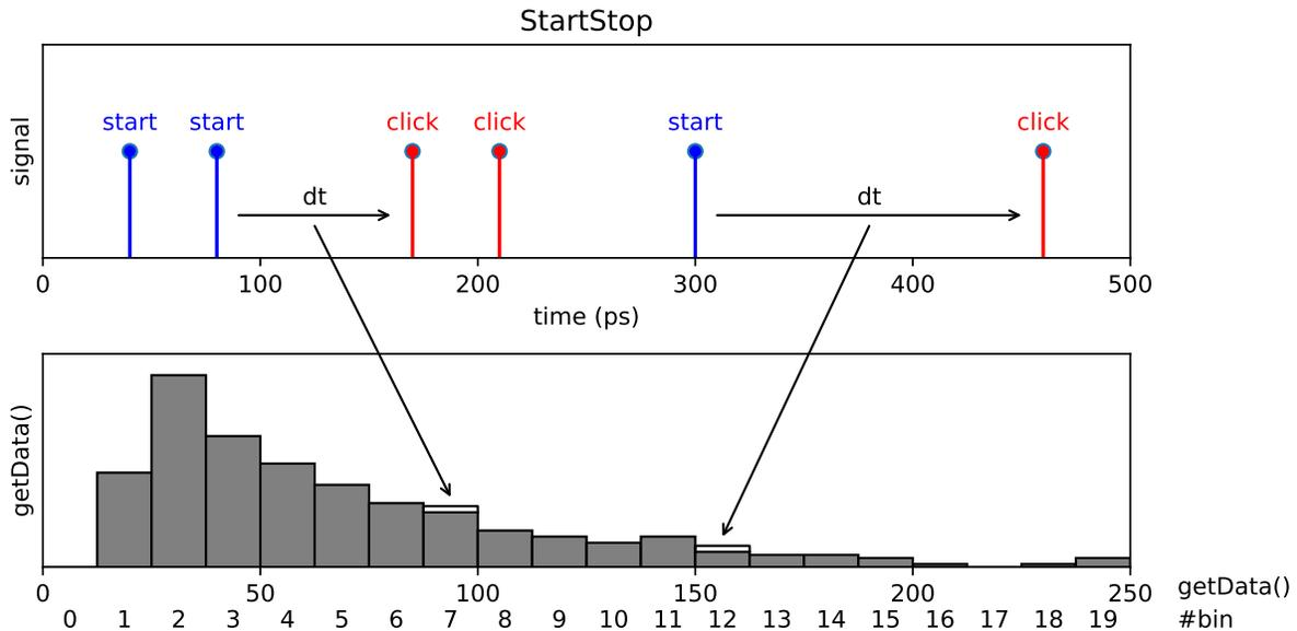
A simple start-stop measurement. This class performs a start-stop measurement between two channels and stores the time differences in a histogram. The histogram resolution is specified beforehand (*binwidth*) but the histogram range (number of bins) is unlimited. It is adapted to the largest time difference that was detected. Thus, all pairs of subsequent clicks are registered. Only non-empty bins are recorded.
