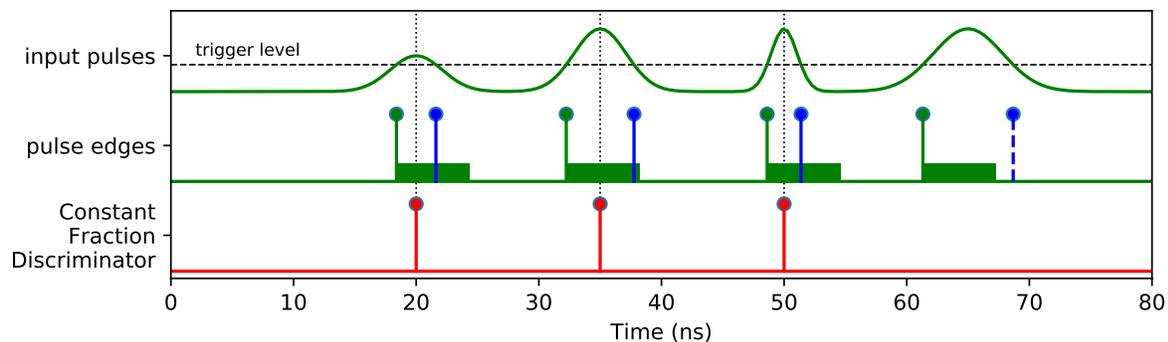
Constant Fraction Discriminator (CFD) detects rising and falling edges of an input pulse and returns the average time of both edges. This is useful in situations when precise timing of the pulse position is desired for the pulses of varying durations and amplitudes.
