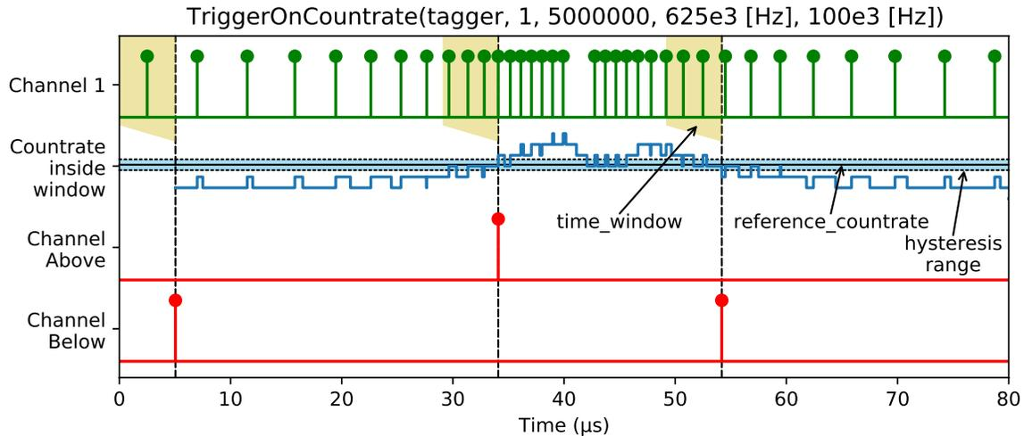
The time-tags are always injected at the end of the integration window. You can use the `DelayedChannel` to adjust the temporal position of the trigger tags with respect to the integration time window.
