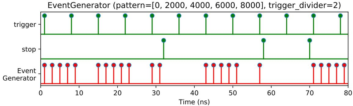
Emits an arbitrary pattern of timestamps for every trigger event. The number of trigger events can be reduced by *trigger\_divider*. The start of a new pattern does not abort the execution of unfinished patterns, so patterns may overlap. The execution of all running patterns can be aborted by a click of the *stop\_channel*, i.e. overlapping patterns can be avoided by setting the *stop\_channel* to the *trigger\_channel*.
