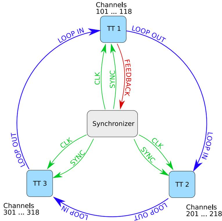
**Warning:** For reliable synchronization, the cables for *CLK* and *SYNC* signals shall have a length difference below 4 cm. We recommend using the same cable type for these two signals.
