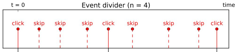
Applies an event divider filter with the specified factor to a channel, which reduces the data rate. Only every  $n$ -th event from the input stream passes through the filter, as shown in the image. The divider is a 16 bit integer, so the maximum value is 65535.
