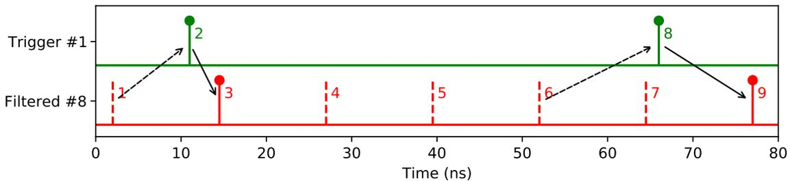
The dashed line indicates which pulse excited the sample. If the photon is emitted early by the sample (click 2), it will trigger the first pulse (click 3) after the stimulating one (click 1). In the second case, the photon is emitted late and the subsequent laser pulse (click 7) has already passed. In this case, click 9 is passed and click 8 seems to be very early, although it is quite late, in fact.
