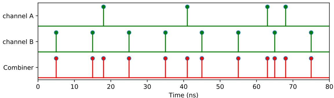
Combines two or more channels into one. The virtual channel is triggered, e.g., for two channels when either channel A OR channel B received a signal.
