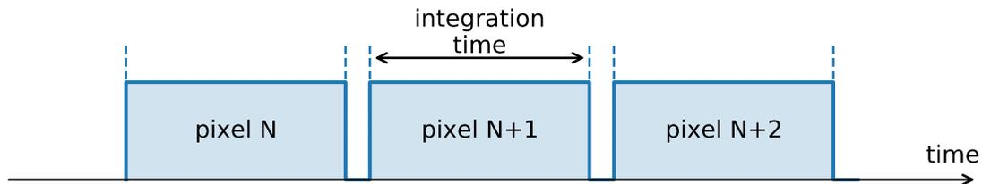
The case when the pulse width defines the integration time has been considered in the previous subsections.
