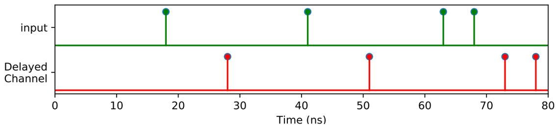
Clones input channels, which can be delayed by a time specified with the `delay` parameter in the constructor or the `setDelay()` method. A negative delay will delay all other events.
