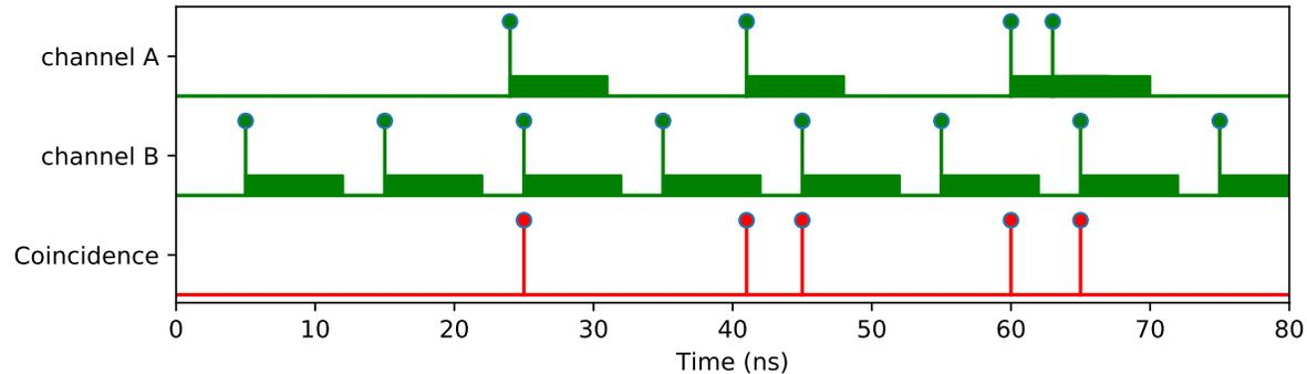
Detects coincidence clicks on two or more channels within a given window. The virtual channel is triggered, e.g., when channel A AND channel B received a signal within the given coincidence window. The timestamp of the coincidence on the virtual channel is the time of the last event arriving to complete the coincidence.
